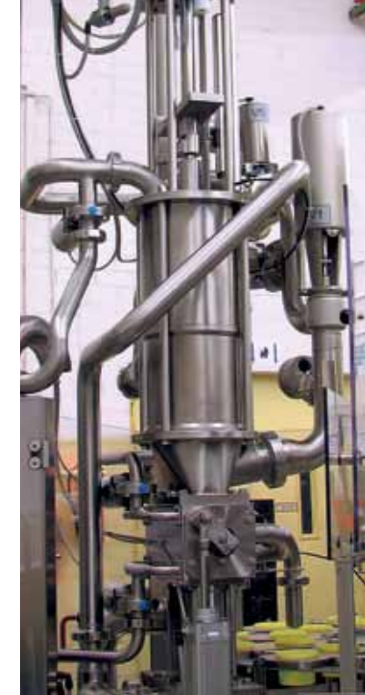
Compensation cylinder for synchronizing continuous product feed and discontinuous filling process
