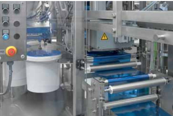
Roll stock sealing station with wind-up of remaining foil, and without pressure/squashing of the bucket structure during sealing.
