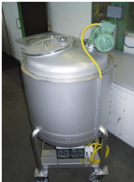
Mobile container, with agitator, electric heating mats with temperature control and insulation
