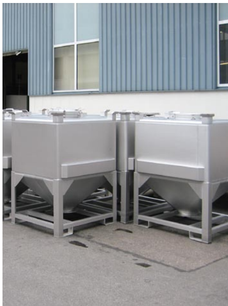
Mixing and turning cubic tank container, for asymmetric moved mixer
